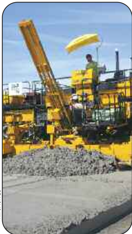
The frame-mounted tie bar inserter (TBI) accurately places the transverse bars for the longitudinal joint by placing the bars behind the vibrators.
