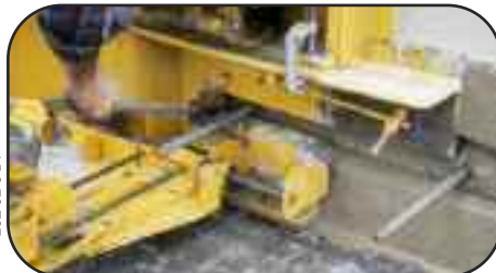
Female keyway with hydraulic side bar insertion (SBI) and vibration to the bar.
