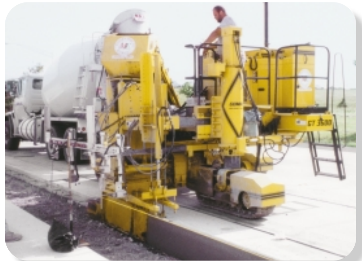
The GT-3600 (above photo) with All-Track Positioning (ATP) provides easy set up for slipforming sidewalk or (below photo) curb and gutter to the existing slab. Steering and grade is referenced off the existing curb or can be referenced off the stringline.
