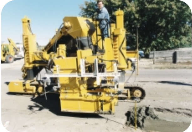
This GT-3600 has a Guillotine-style curb depressor.
