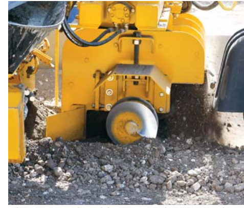
The trimmerhead has more than enough power to trim through crushed gravel base.
