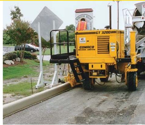
Optional rubber tires are available instead of the gear-driven crawler tracks.
