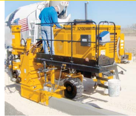
The rubber tires have a travel speed of 107 feet per minute (32.6 mpm).
