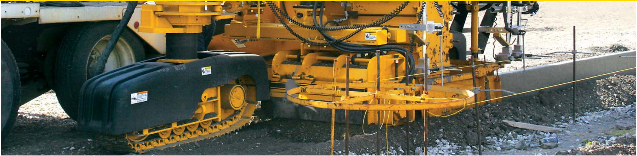
The front-steer capable GT-3200 with All-Track drive will slipform a 24 inch (610 mm) radius. The front leg design has more steering torque for tighter turning capabilities and maneuverability.
