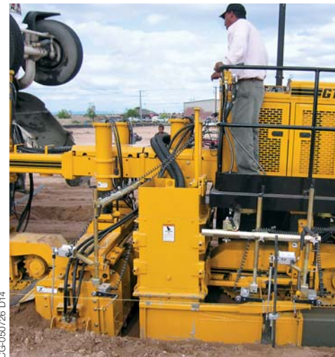
The front-steer capable GT-3200 with All-Track drive will slipform a 24 inch (610 mm) radius. The front leg design has more steering torque for tighter turning capabilities and maneuverability.
