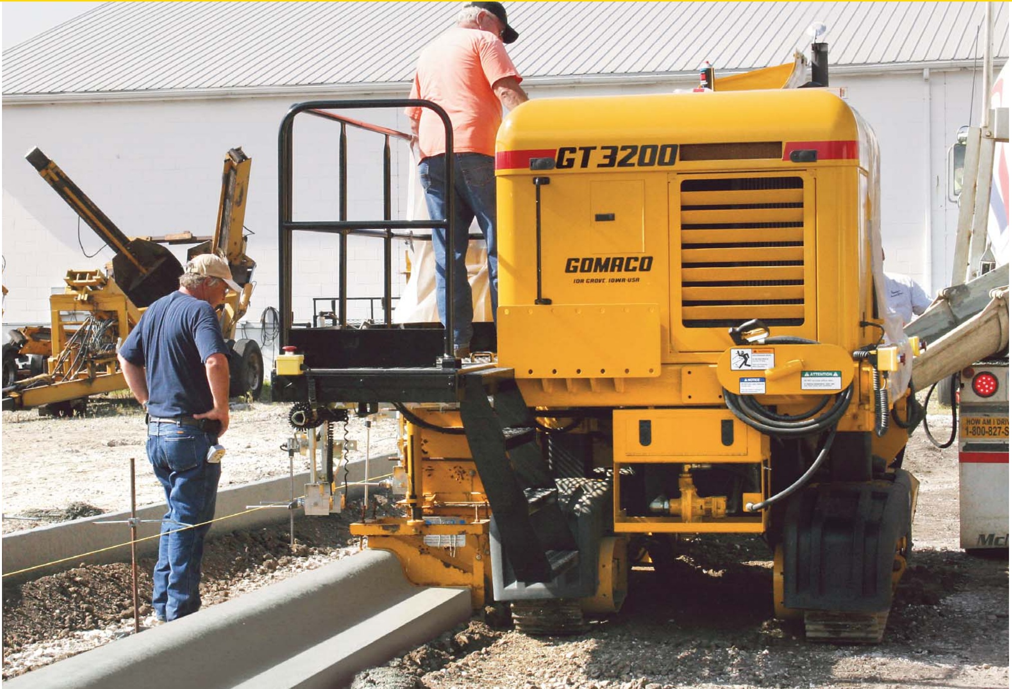
The molded fiberglass shroud on the GT-3200 is lightweight and provides easy access to the engine and other components. Overall width of the machine is only 8.5 feet (2.59 m).
