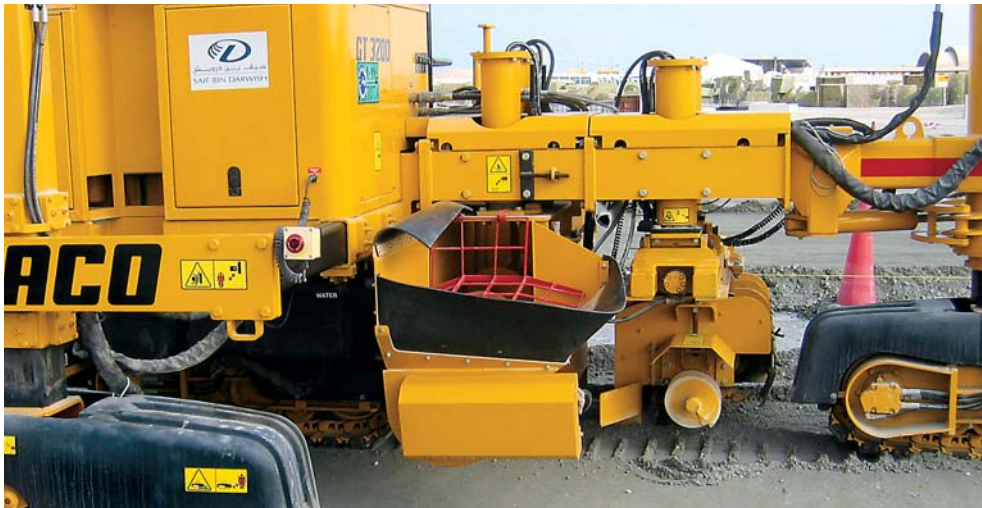
The front-steer capable GT-3200 with All-Track drive will slipform a 24 inch (610 mm) radius. The front leg design has more steering torque for tighter turning capabilities and maneuverability.
