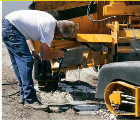
The auger features a latched clean-out door at the receiving end of the hopper.
