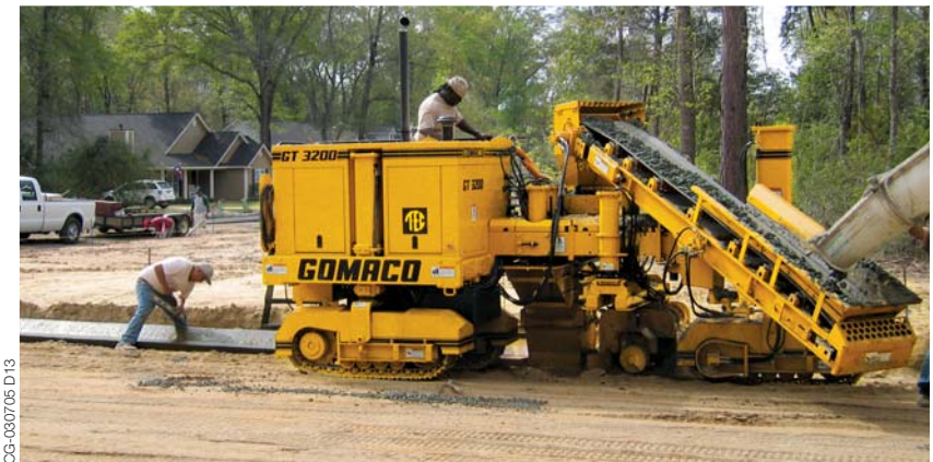
An optional 13.5 foot (4.1 m) long conveyor is available instead of an auger.
