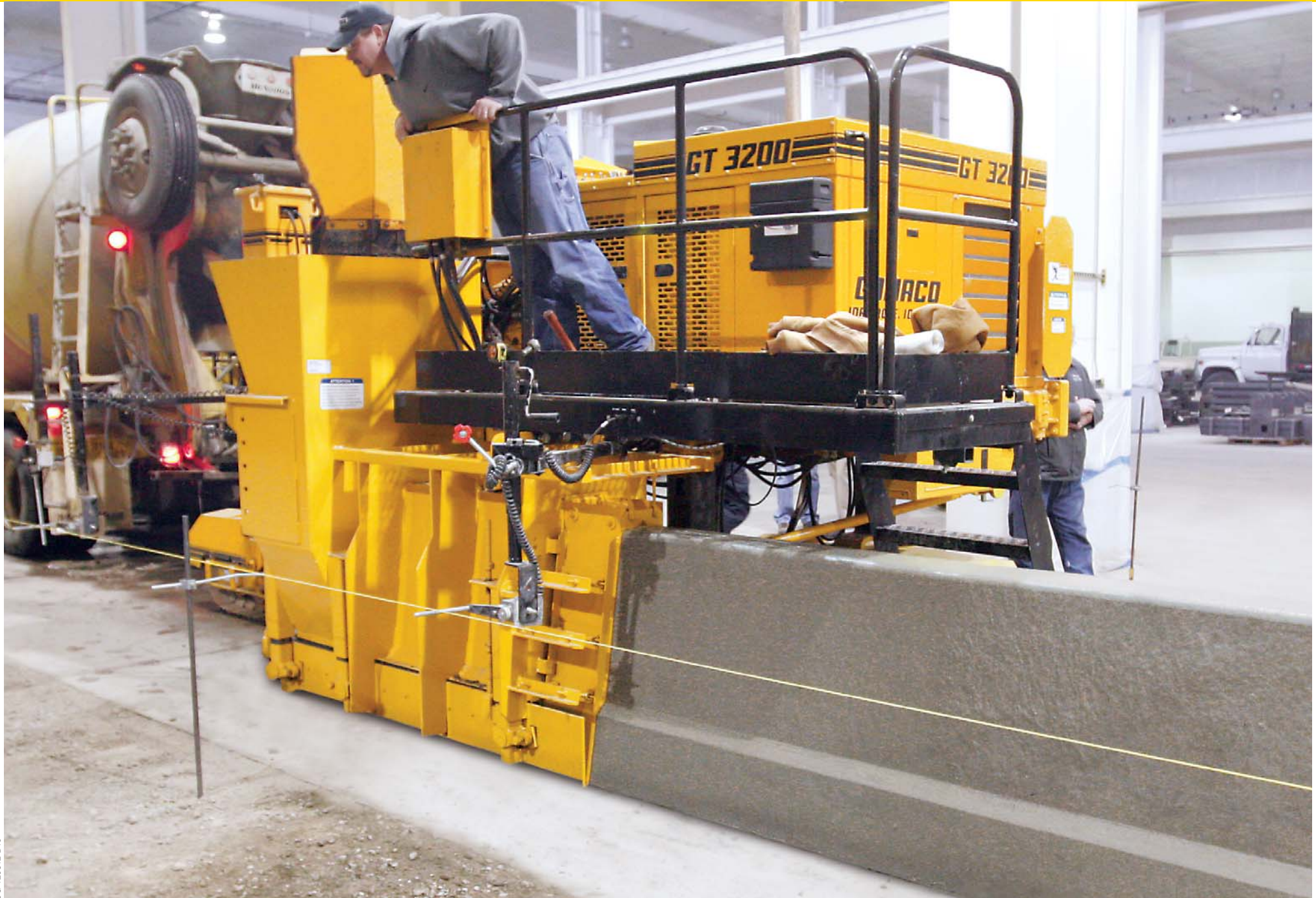
The GT-3200, with an optional high-volume conveyor, can slipform right-side or left-side barrier wall up to 40 inches (1016 mm) tall.
