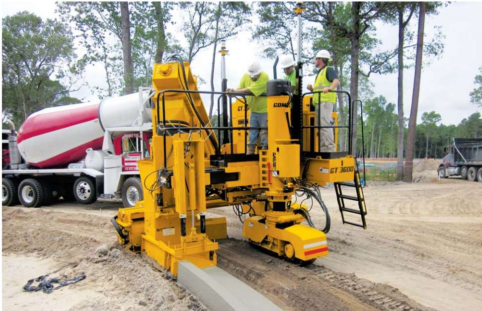
Repeatable mold offset is accomplished through G+ and a smart hydraulic cylinder for telescoping the mold mounting system.
