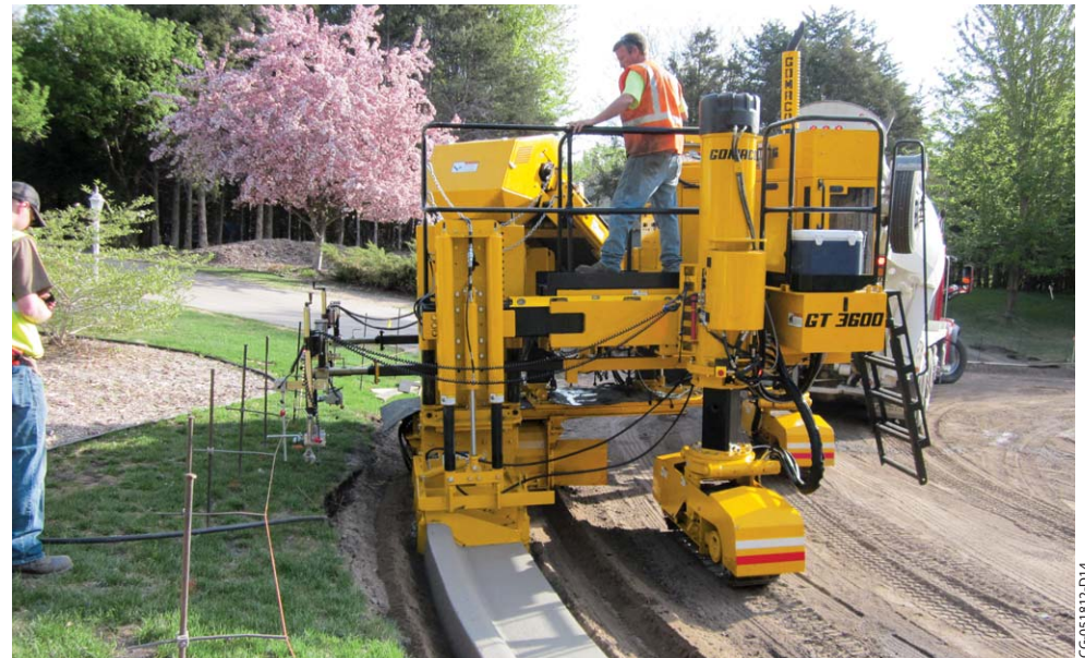
The exclusive independent adjustable stainless steel troweling section at the end of the curb and gutter mold seals and provides a superior GOMACO finish.
