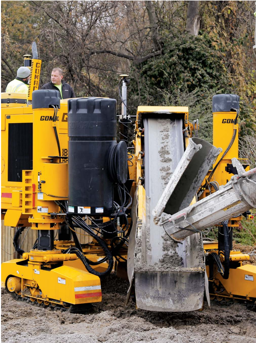
The Xtreme GT-3600 is equipped with a 15 foot (4.6 m) long, 24 inch (610 mm) wide conveyor to move the concrete into the hopper at a speed of up to 284 feet per minute (86.6 mpm).
